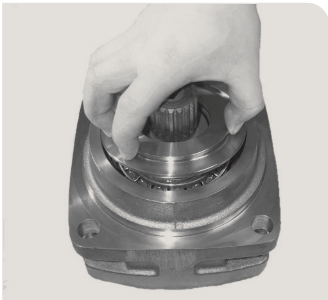
7. Assemble the seal ring carrier with shaft seal.
