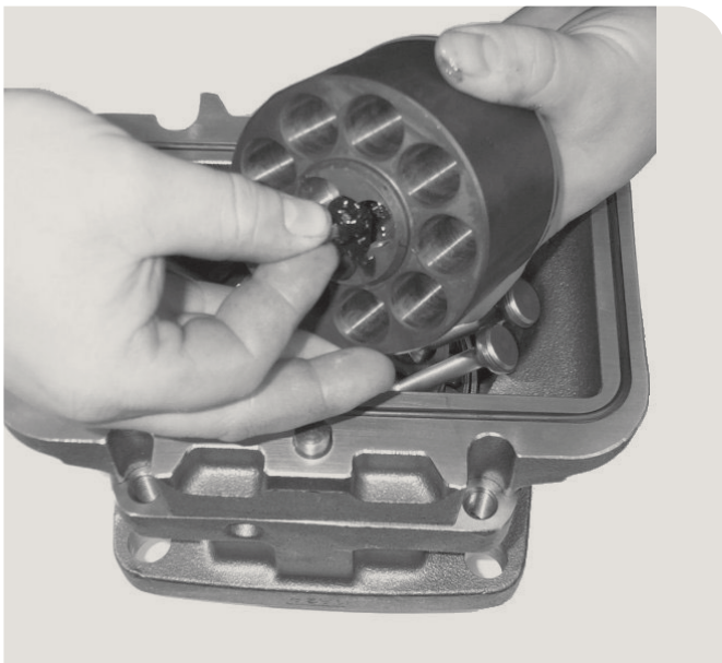
15. Assemble the upper support pin in the cylinder barrel. Put some grease on the pin so it don't fall down when assembling the cylinder barrel.
