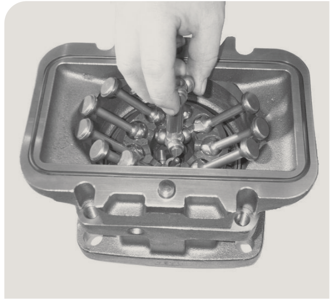
14. Assemble the joint shaft. Put some grease on the joint shaft so the rollers don't fall off.
