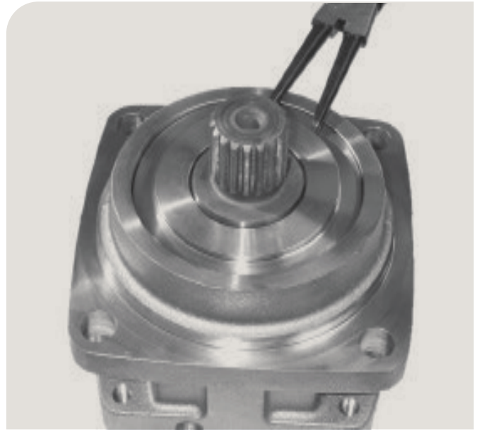
14. Remove the seal carrier with shaft seal off. Change the shaft seal. Use the old shaft seal and press down the new shaft seal into the seal carrier.
