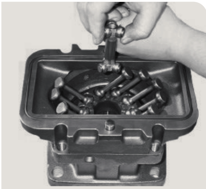
7. Remove the joint shaft. Make sure all joint rollers follow.
