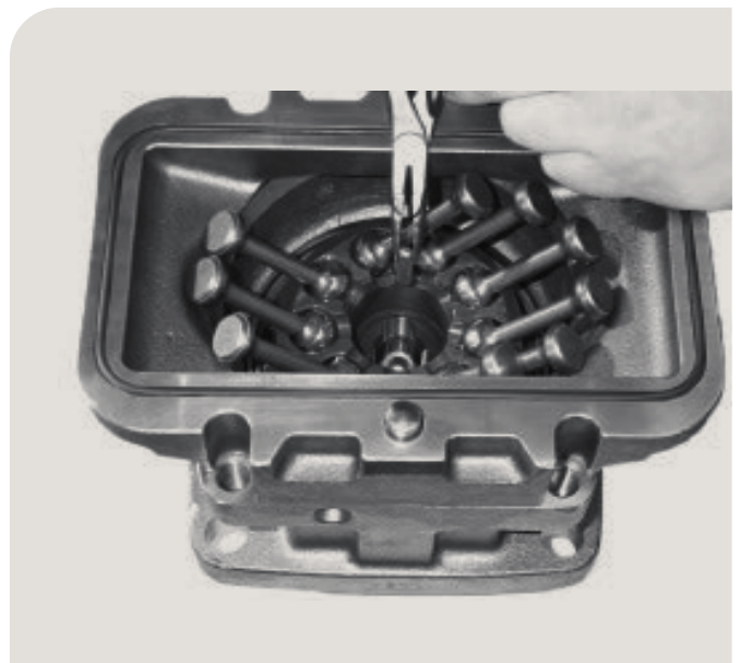
8. Remove the support pin assembled between joint shaft and guide pin.
