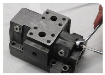
20. Assemble the adjusting screw and seal nut.
