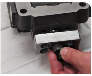
39. Assemble the cover assy. Make sure not to damage the O-ring.
