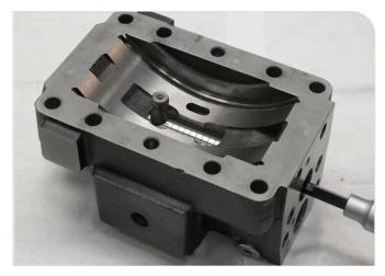
24. Torque the set screw to 14±4 Nm.
