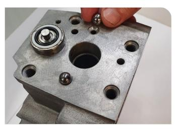
35. Assemble the check valve balls.
