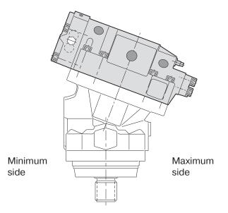
HO and HP control shold be assembled with the control cover at the minimum side.
