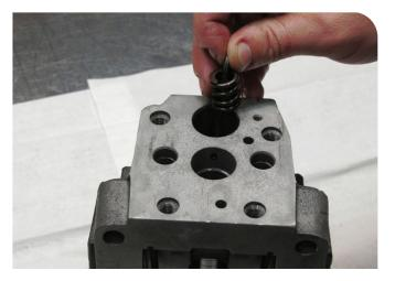
30. Assemble the threshold spring.
