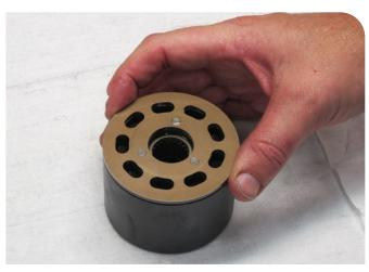
10. Assemble the sliding plate.
