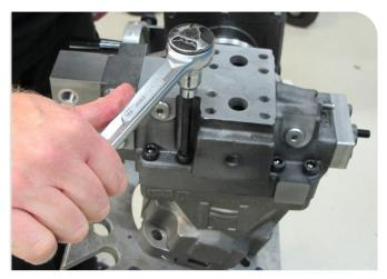
54. Assemble the screws and torque the screws to  $65\pm10$  Nm for V12-60/80 and  $105\pm20$  Nm for V12-110/160.
