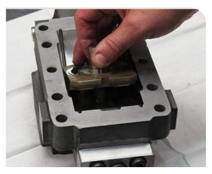
41. Assemble the valve segment in the end cap. The slot in the valve segment against the cover side.
