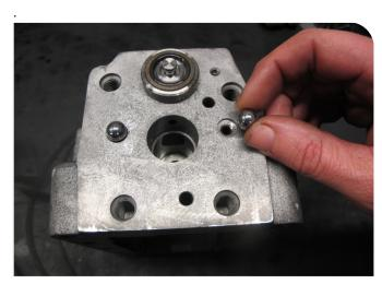
B. Assemble the check balls.
