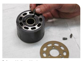
9. Assemble the guide pins.
