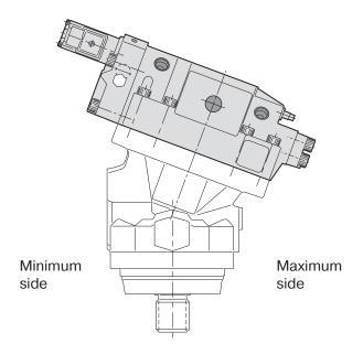
EO and EP control shold be assembled with the control cover at the minimum side.
