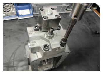
C. Assemble the control cover and torque the screws to  $65\pm10$  Nm for V12-60, -80 and -110.  $105\pm20$  Nm for V12-160.
