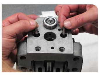
34. Assemble the valve cones.
