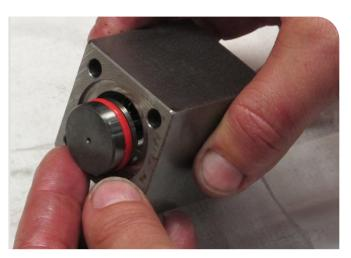
14. Assemble the control piston in the AH-housing.
