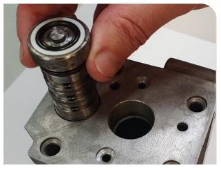
33. Assemble the valve sleeve assy. Make sure the spool hits the guide hole in the spring seat.
