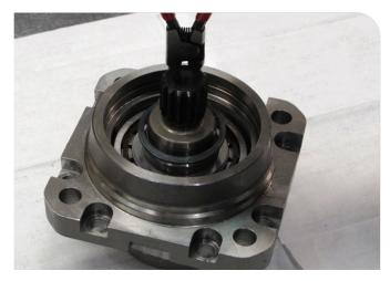
5. Assemble the retaining ring. Make sure it is all the way into the groove. Check the pre-load of the bearings, not to tight and no back-lash.
