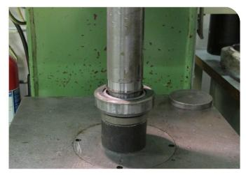
1. Press down the big tappered roller bearing and the inner ring for the roller bearing in two steps.
