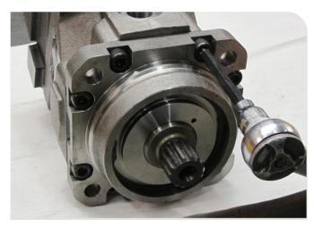
55. Assemble the screws and torque the screws to  $65\pm10$  Nm for V12-60/80 and 105±20 Nm for V12-110/160.
