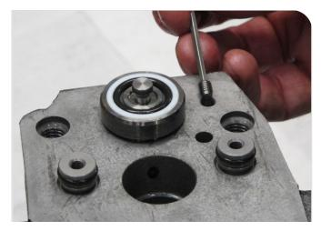
36. Assemble the nozzles and torque them to 1,2±0,2 Nm.
