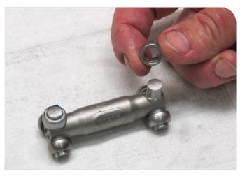
11. Assemble the joint rollers on the joint shaft. Make sure the step on the joint rollers is fitted inwards.
