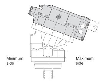
AC and AH control shold be assembled with the control cover at the maximum side.
