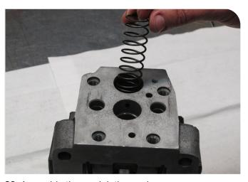
28. Assemble the modulating spring.
