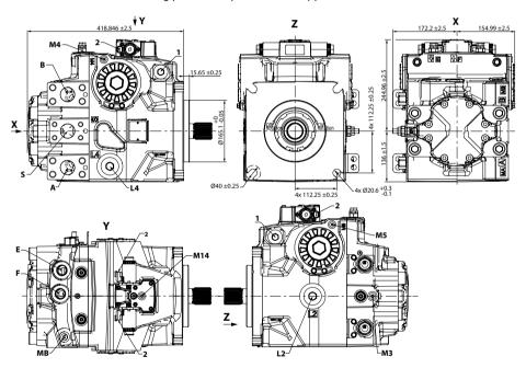
${\bf A/B}$  system ports: Ø38 mm, 450 bar split flange boss per ISO 6162, M16 x 2; 27 min. full thread depth
