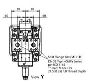
DIN ISO 3019/2 with Electric Proportional Control (de-energized = min. displacement)
