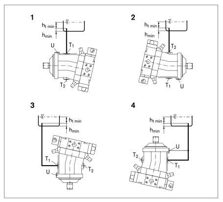
Fig. 6: A6VM below-reservoir installation - A6VM with installation position 1-4
