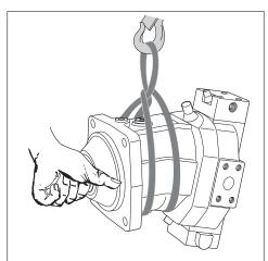
Fig. 5: Transport with lifting strap
