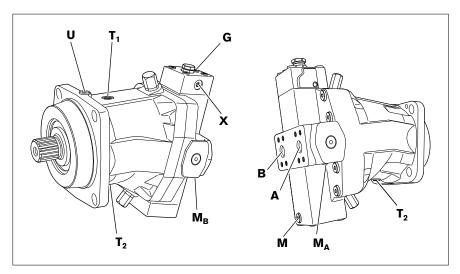
Fig. 14: Port overview of A6VM 250-1000 HD, service line ports at rear
