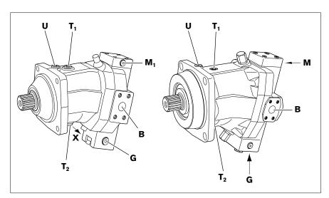
Fig. 17: Port overview of A6VM 28-200 HA (left), A6VM 250-1000 HA (right), service line ports at side
