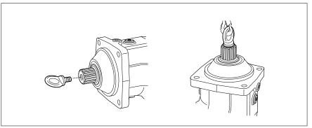
Fig. 4: Fixing the ring screw
