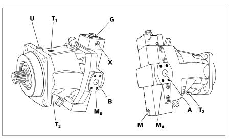
Fig. 13: Port overview of A6VM 250-1000 HD, service line ports at side
