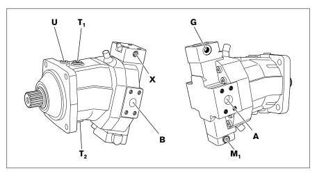
Fig. 11: Port overview of A6VM 28-200 HD, service line ports at side
