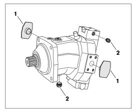
Fig. 9: Removing transport protection
