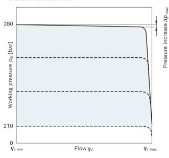
Characteristic curve valid for  $n_1$  = 1500 rpm and  $t_{fluid}$  = 50 °C.
