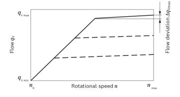
Characteristic curves valid for  $n_1$  = 1500 rpm and  $t_{fluid}$  = 50 °C.
