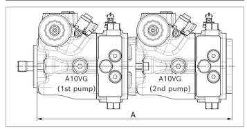
By using combination pumps, it is possible to have independent circuits without the need for splitter gearboxes.
