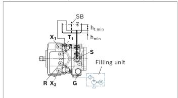
Recommendation: Filling with filter/filling unit.
